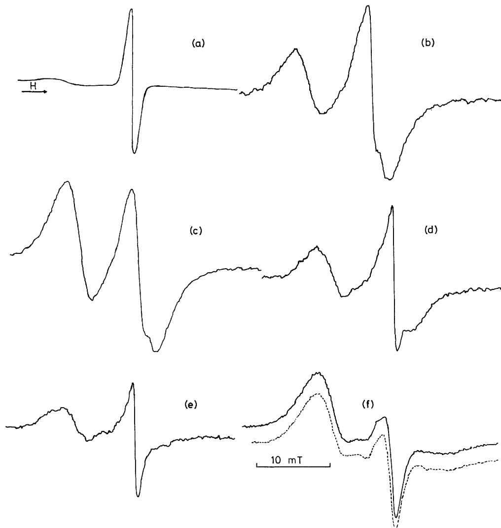
Figure 1. E.s.r. spectra (9.1–9.2 GHz) of \gamma -irradiated (77 K) alkali metal hydroxide ( ca. 10 M) aqueous glasses at 77 K. (a) KOH, microwave power 10^{-2} mW; (b) RbOH, microwave power 10^{-2} mW; (c) RbOH, microwave power 2 mW; (d) RbOH after a brief period of photobleaching ( \lambda > 340 nm; 15 s); (e) RbOH after a further period of photobleaching ( \lambda > 340 nm; 50 s); (f) CsOH, microwave power 10^{-2} mW, before (—) and after (---) prolonged photobleaching.
